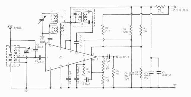
Fig. 1. Circuit diagram of the radio tuner.
