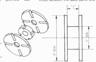
Fig. 4. Suggested construction of former for winding coils L1, L2 and L3. Wooden former is held together by centre bolt – here removed. Any suitable construction may however be used providing dimensions follow drawing on right.
