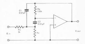
A simple bandpass filter may be constructed using an op-amp and a few discrete components. The circuit shown has a constant gain and bandwidth, and the centre frequency may be adjusted from 1.6 kHz to 2.4 kHz by changing Rc from 1100 ohms to 400 ohms. Gain is 26dB at centre frequency and bandwidth is 775 Hz at 10dB down.
