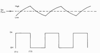
Fig. 2. Operation of thermostat above and below set point, upper curve shows temperature of load, lower curve shows heater being turned on and off.
