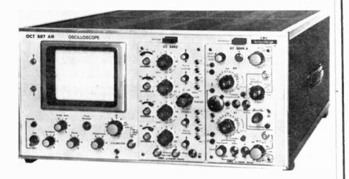
To meet the need for an oscilloscope which would trigger directly from PAL colour signals Schlumberger CRC have released the BTV 5851 plug-in time base for their OCT 587 and 588 series oscilloscope main frames.
