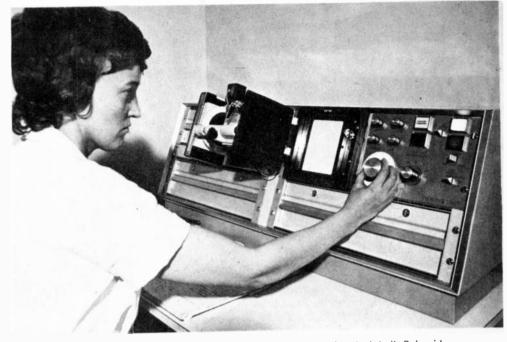
Viewing unit. Results may be examined directly or photographed using the inbuilt Polaroid Land camera.
