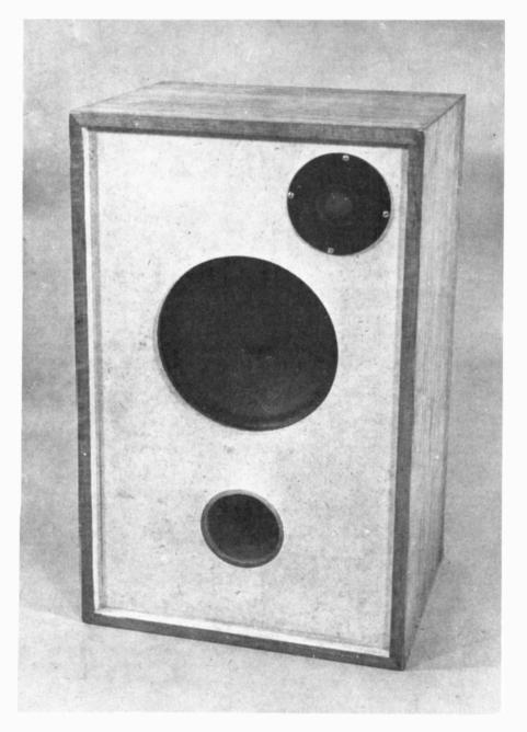
The completed speaker without the front grille fitted.
