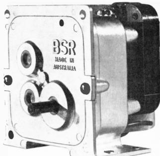
The VPS100 gear box is designed for applications re-quiring a compact, powerful drive unit and features a die-cast housing, sintered bronze bearings; machine-cut steel gears and pinions plus a non-metallic gear in the first reduction to keep noise to a minimum.
