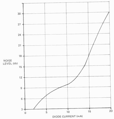
noise output, say twice the value just measured, and note the potentiometer dial setting. The front-end of the radiometer, particularly the input tuning and matching, is then adjusted such that the same noise increase is attained with successively lower amounts of current flowing through the diode after each adjustment to the receiver's circuitry is made. Never make more than one change at a time.
