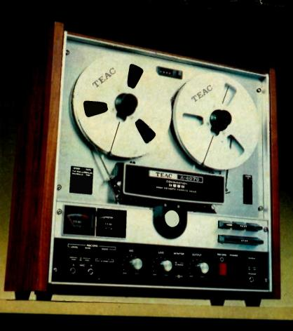
Bi-directional record and playback tape deck Model A-4070 ● 4 Ferrite heads (6 head function) ● Reel size 7" ● Tape speed 3<sup>3</sup>4 ips and 7<sup>1</sup>/<sub>2</sub> ips ● Triple motor mechanism ● Wow and flutter .06% at 7<sup>1</sup>/<sub>2</sub> ips ● F/R 25 to 24,000 Hz at 7<sup>1</sup>/<sub>2</sub> ips ● S/N ratio 58dB
