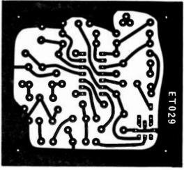
Fig. 3. PC board layout for the tuner (full size)
