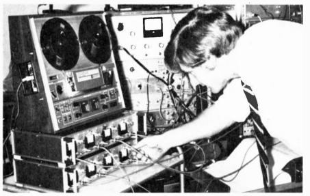
An Australian designed and built eight channel analogue recording system has recently been introduced by Electrodata Associates Pty. Ltd. The model MT465 system incorporates the use of multiplex techniques to record two analogue channels on each tape track. As a consequence, the system incorporates a four track, ¼ inch tape deck thus enabling its cost to be held at less than one-half of other eight channel systems.
