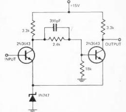
By replacing the common-emitter resistor in a conventional Schmitt by a zener diode, the hysteresis normally associated with these circuits is eliminated.
