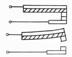
Fig. 1. Basic thermostat: when heated, brass (shaded) portion expands more than invar thus causing strip to bend and contact to open.
