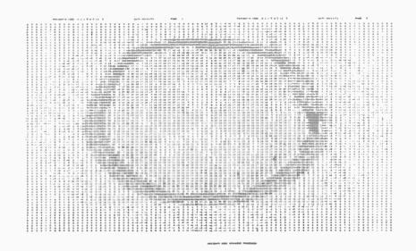
In addition to the pictures produced on the cathode ray tube viewing unit, the results of the X-ray scans may be printed out by computer. This numerical print-out shows the absorption coefficients of the material at each point, providing detailed information on the atomic number and density of the tissue at each picture matrix point.
