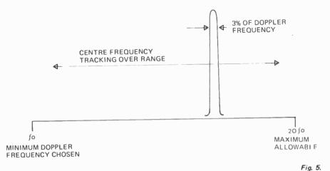
tracking filters. By this approach the quality of the doppler frequency bursts are improved enormously.
