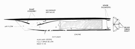
A cross section of engine nacelle of Concorde.
