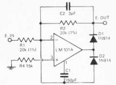
A precision half wave rectifier using an operational amplifier may be constructed as shown. This will have a rectification accuracy of 1% from dc to 100 kHz.
