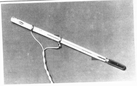
Fig. 4. Basic contact thermometer – designed to switch at  $40^{\circ}$ C. At that temperature, the expanding mercury touches the second contact point.
